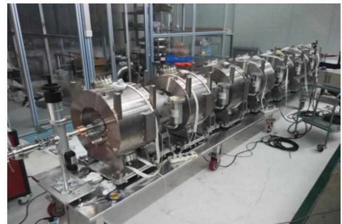
**Seven Spoke012 cavities ready for assembly in CM1**
