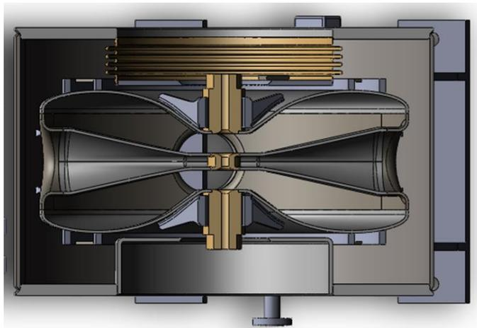
**Cross section of Spoke012 cavity**
