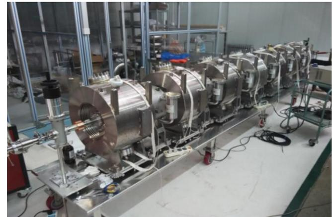
**Seven Spoke012 cavities ready for assembly in CM1**
