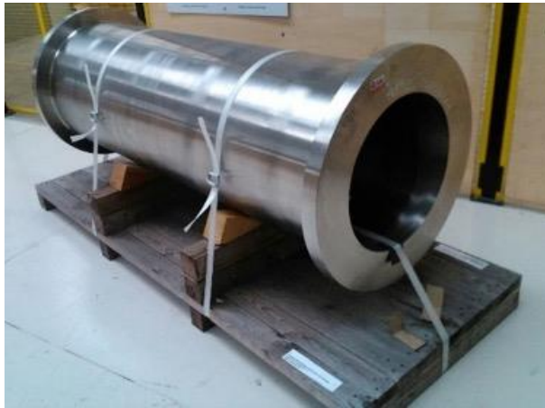
Tank 4: forged 304 L stainless steel
