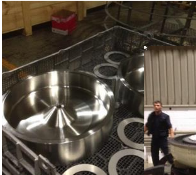
Buncher Cavity Production and Heat Treatment
