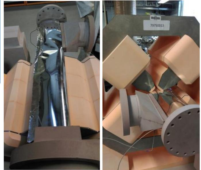
Test shaping insulation coats (aluminum coated PI)
