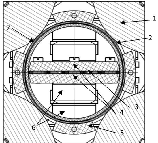
Figure 4: Section view of probe with slide bearing inside yoke. 1 - Yoke, 2 - Bearing frame, 3 - PCB, 4 - Holding plates, 5 - Anchor, 6 - Adjusting inserts, 7 - Probe frame.
