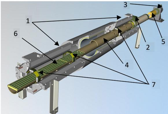
Figure 3: 3D model of the probe installed in the magnet. 1 - Quadrupoles doublet, 2 - Thrusting bracket, 3 - Motor, 4 - Tubular fiberglass frame, 5 - Slip rings, 6 - PCB, 7 - Bearings
