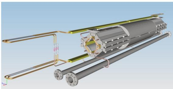
Figure 1: Booster quadrupole magnet.
