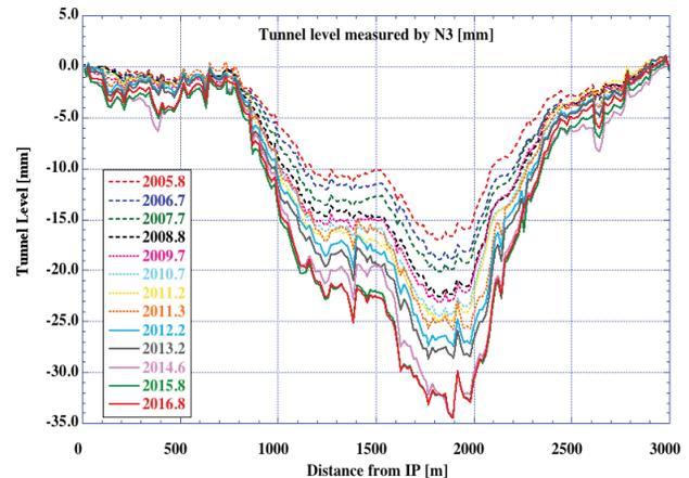
Figure 1: The tunnel level trend from the middle point of the KEKB B-factory accelerator operation to the SuperKEKB phase-1 commissioning. The vertical displacement of the beamline levels along the LER from the interaction point (IP) to the IP.
