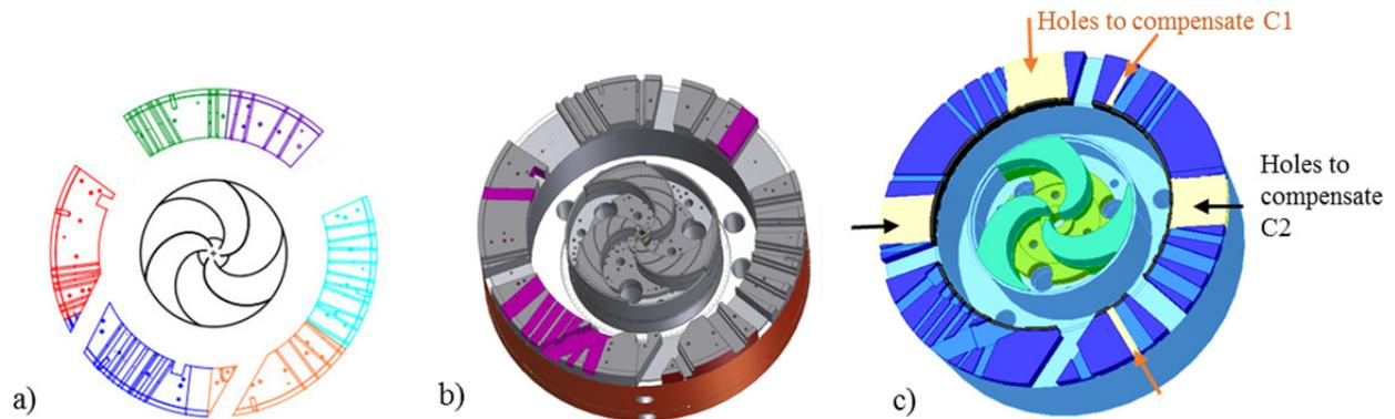
Figure 1: Views of the bottom half of the CS. The first ones, a) and b), are top views of the CS as it is today. In a), the existing extraction channel is in the orange sector. In b) the modifications needed to add the new extraction channel, which is almost 30 degrees away from the old one, are shown in magenta. Finally, c) shows the results of the optimization's process, see text. The arrows highlight the areas where the iron has been removed.
