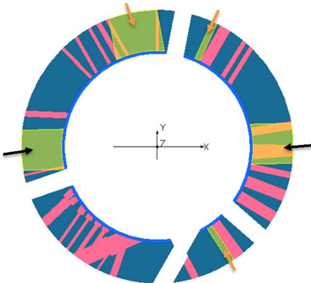
Figure 2: Central iron ring of the yoke of the CS. In navy, there is the iron with all the penetrations needed to guarantee both extraction methods. In translucent yellow, there are the profiles of the new penetrations to add to the central iron ring of the yoke to cancel the first (orange arrows) and second (black arrows) field harmonic components.
