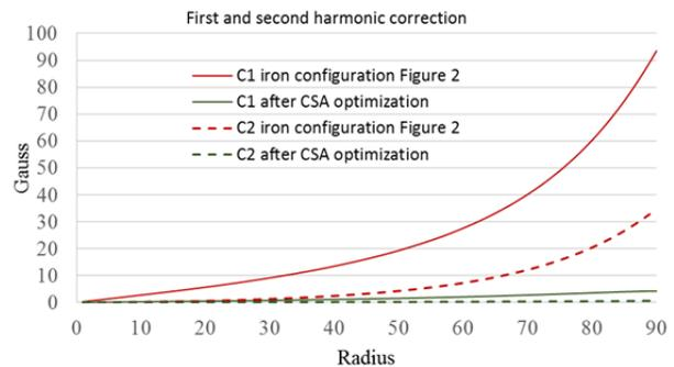
Figure 3: First and second harmonic before and after the optimization process using the CSA method.
