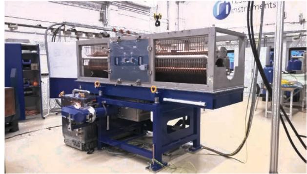
Figure 2: First of Series (FOS) SIS100 acceleration cavity at factory acceptance test at Research Instruments.
