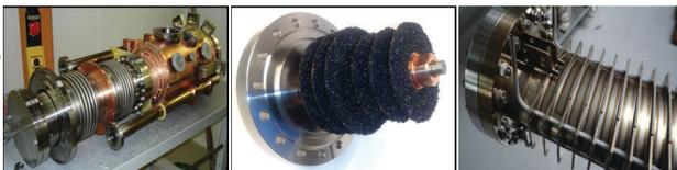
Figure 4: Cryogenic pumping of the UHV system in SIS100. Left a cryocatcher, in the middle a cryosorption pump and right a cryogenic magnet chamber.
