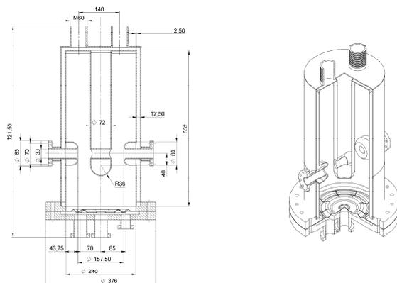
Figure 5: General view of 162 MHz QWR for  $\beta_G = 0.12$ , RF load loop and measurement loop are not seen.
