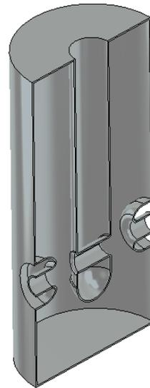
Figure 4: General view of 162 MHz QWR for  $\beta_G = 0.12$ .
