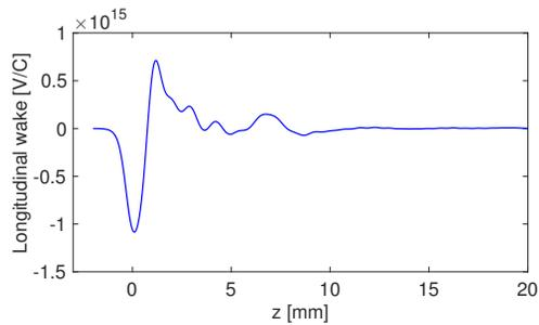
Figure 3: ALS-U longitudinal pseudo-Green computed with CST Particle Studio and  $\sigma=0.3$  mm.
