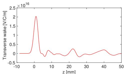
Figure 5: ALS-U transverse pseudo-Green function computed with CST Particle Studio and  $\sigma=1$  mm.
