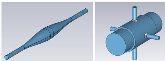
Figure 2: 3D models used for CST impedance simulations of the large ID BPM (left) and the small ID taper transition (right). The models are not to scale.
