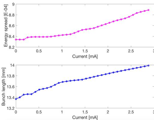
Figure 4: ALS-U energy spread and bunch length as a function of the beam current, computed with Elegant using the short range longitudinal wake and RW impedance as input.
