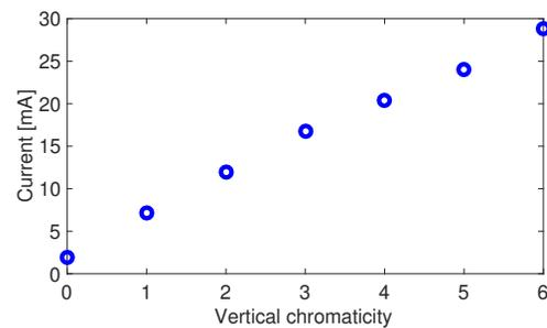
Figure 6: ALS-U TMCI threshold current as a function of the vertical chromaticity, computed with Elegant using the short range transverse wake and RW impedance as input.
