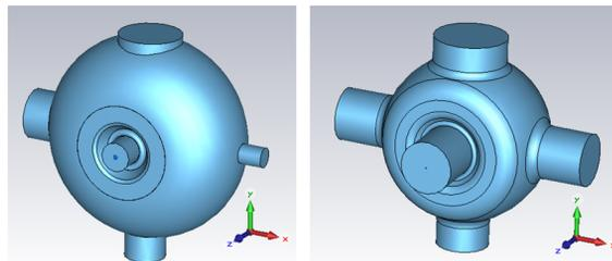
Figure 1: 3D models used for CST impedance simulations of the main cavity (left) and harmonic cavity (right).
