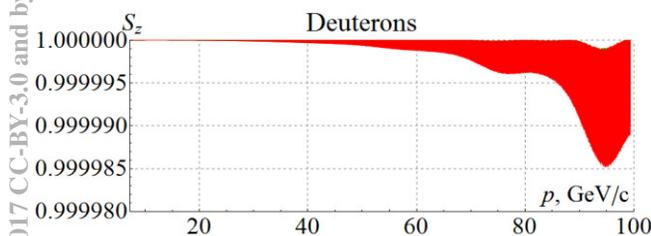
Figure 7: Longitudinal spin component during acceleration of three deuterons in the ion collider ring.
