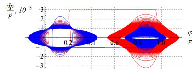
Figure 8: Proton phase space trajectories.
