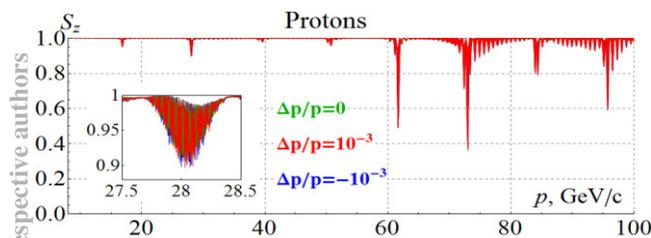
Figure 6: Longitudinal spin component during acceleration of three protons in the ion collider ring.
