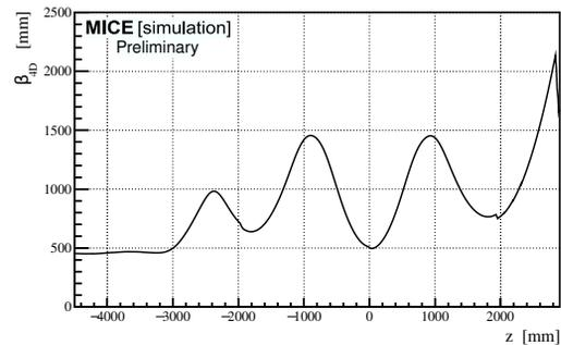
Figure 7: Evolution of the transverse betatron function for the 200 MeV/c setting in the simplified lattice. Significant growth can be seen, following the secondary absorber at  $z = 2000\text{mm}$ , due to the lack of magnetic fields.
