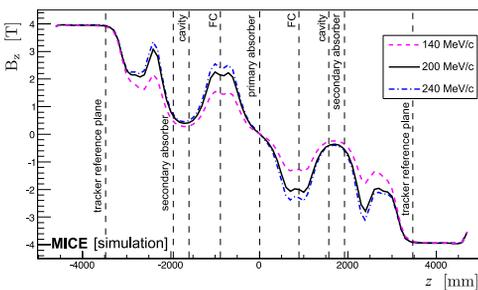
Figure 2: Longitudinal magnetic field strength through the length of the cooling channel for the 200 MeV/c (solid black line), 140 MeV/c (dashed purple line) and 240 MeV/c (mixed blue line) settings. The position of key components are indicated by the vertical lines.
