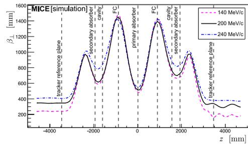
Figure 3: Transverse betatron function through the length of the cooling channel for the 200 MeV/c (solid black line), 140 MeV/c (dashed purple line) and 240 MeV/c (mixed blue line) settings. The position of key components are indicated by the vertical lines.
