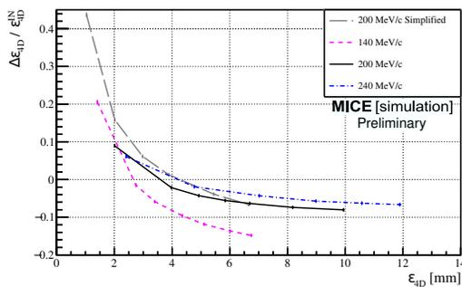
Figure 5: The fractional change in transverse emittance for each transmitted beam as simulated for each emittance of the three momenta settings. The 200 MeV/c setting for the simplified design is also included for comparison.
