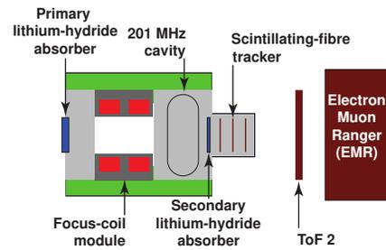
Figure 6: Layout of the downstream components of the simplified design. The spectrometer solenoid has been replaced by a 3-station tracker and the KL detector has been removed to improve the momentum resolution.
