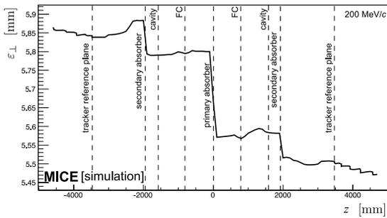
Figure 4: Evolution of the transverse emittance for a transmitted 6 mm beam, with central momentum 200 MeV/c (RMS spread 4.0%). The position of key components are indicated by the vertical lines.
