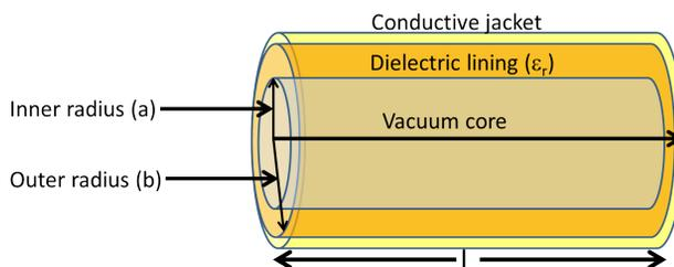
Figure 1: A cylindrical dielectric-lined waveguide (DLW) with dimensions  $(a, b, \epsilon_r, L)$  is illustrated. The region  $r < a$  is vacuum,  $a < r < b$  is filled with dielectric material with relative permittivity  $\epsilon_r$  and the outer radius is coated with a conductor. The length of the structure is  $L$ .
