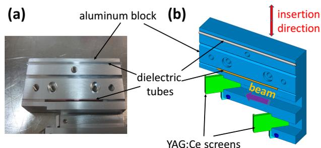
Figure 3: Picture (a) and schematic (b) of the DLW holder designed and built for PITZ. Here several tubes were mountable and YAG:Ce screens were used for beam-alignment. The mount was placed in an actuator for vertical alignment; horizontal and angular alignments were done upstream with beam steerers.
