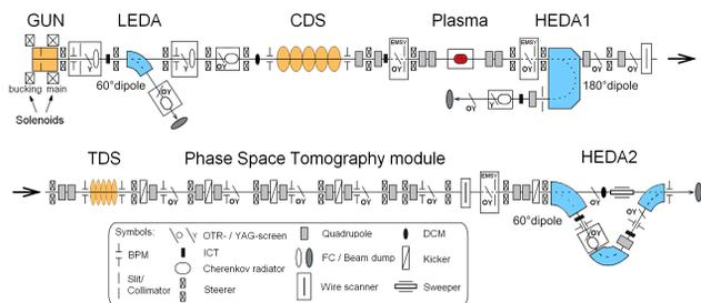
Figure 2: Experimental layout of the PITZ photoinjector. The acronyms "LEDA", "CDS", "HEDA" and "TDS" respectively refer to the "low energy dispersive area", "cut-disk structure", "high-energy dispersive area", and "transverse-deflecting structure".
