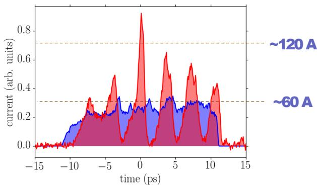
Figure 4: Current profile with (red trace) and without (blue trace) the  $\lambda=1.03$  mm DLW; head of the bunch is on the left side i.e. negative time. The peaks are consistent with the wavelength of the structure  $\sim 3.3$  ps. The asymmetric bunching is due in part by the non-rectangular current profile and also from any curvature within the bunch bunch.
