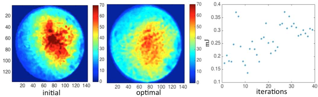
Figure 2: Left: initial beam profile corresponding to  $175\mu\text{J}$ . Middle: optimal beam profile corresponding to  $372\mu\text{J}$ . Right: gas detector reading evolution through 40 iterations.
