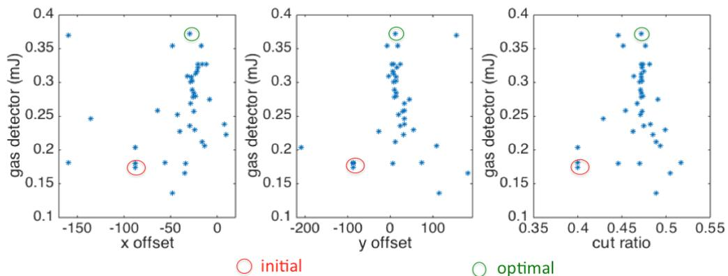
Figure 3: The evolution of the FEL gas detector reading as a function of each of the variables.
