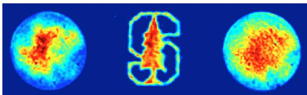
Figure 1: Laser shaping results using DMD. Left: original beam profile. Middle: Stanford tree. Right: cut-Gaussian profile. Note that the color scale of the middle and right images is adjusted to be 60% of the original beam image to show better contrast.
