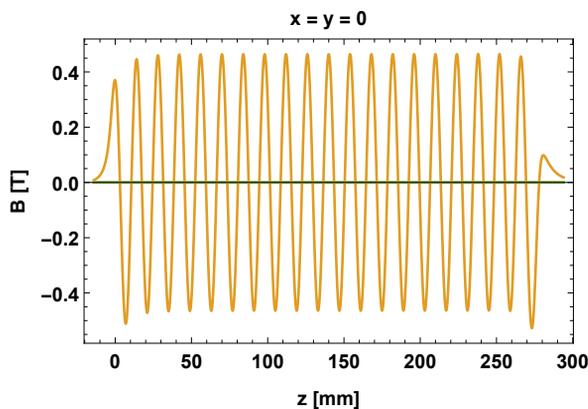
Figure 1: Longitudinal variation of the on-axis, undulator magnetic field components (RADIA simulation). The only non-zero component is the vertical field (brown line).
