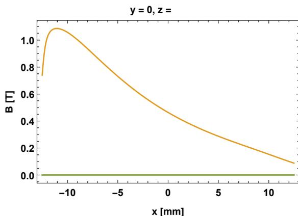
Figure 2:  $x$ -dependence of the median-plane ( $y = 0$ ) magnetic field components (RADIA simulation). The  $z$ -location corresponds to a crest of the  $y$ -field. Once again, the brown line corresponds to the vertical field.
