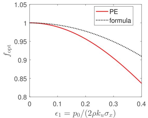
Figure 2: Ratio of the perturbed growth rate vs its unperturbed value (optimized with respect to the detuning  $\hat{\nu}$ ) as a function of  $\epsilon_1$ . Values from the periodic analysis (PE) and the Tanaka formula are included.
