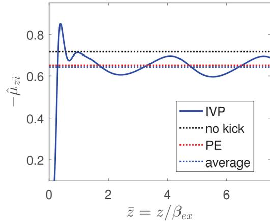
Figure 1: Evolution of the local power growth rate along the undulator. Also included are its average value, the unperturbed growth rate and the result of the periodic analysis.
