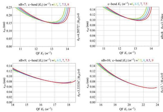
Figure 1: Natural emittance as a function of the arc-cell focusing quadrupole gradient for MBA lattices with  $M = 7, 8, 9$  and  $10$  bending magnets per sector.
