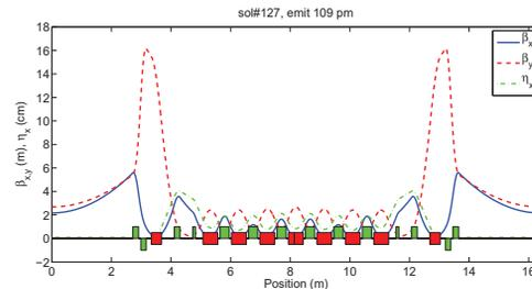
Figure 3: Optics functions for one of the twelve 9-Bend Achromat superperiods.
