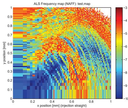
Figure 4: Frequency map analysis at the center of straight. The skew quad amplitude error  $5 \times 10^{-4}$  and normal quad gradient error  $2 \times 10^{-4}$  are included in the lattice.
