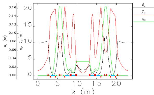
Figure 3: Twiss functions for one DTBA cell in SPS-II.
