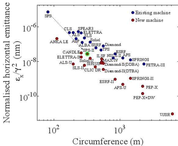
Figure 1: Normalized horizontal beam emittance of existing and planned storage rings.
