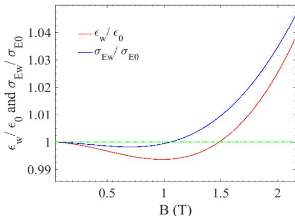
Figure 6: Variation of emittance (red) and energy spread (blue) with undulator field strength.
