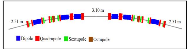
Figure 2: DTBA cell layout.
