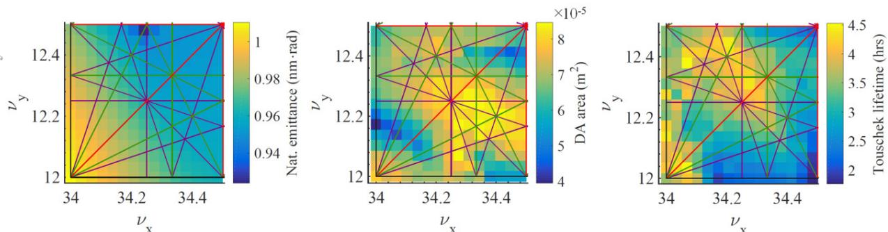
Figure 4: Tune scan results showing natural emittance, dynamic aperture area and Touschek lifetime. Resonance lines: 1<sup>st</sup> (black), 2<sup>nd</sup> (red), 3<sup>rd</sup> (green), 4<sup>th</sup> (purple).
