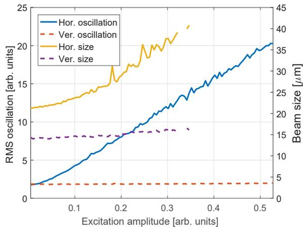
Figure 4: Bunch RMS oscillation and size as function of excitation amplitude. The measurement was conducted at a constant excitation frequency of 115.9 kHz (corresponding to the leftmost peak for this measurement) without any sweep pattern.
