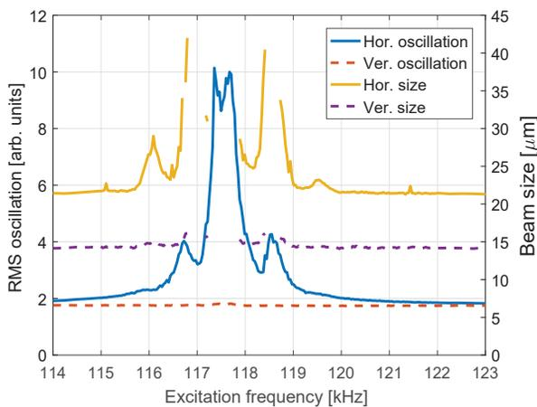
Figure 1: Bunch RMS oscillation and size as function of excitation frequency. In this measurement, the horizontal betatron tune was measured to 117.5 MHz. The measurement was conducted at an excitation amplitude of 0.1.
