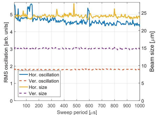
Figure 3: Bunch RMS oscillation and size as function of sweep period. The measurement was conducted at a constant excitation frequency of 115.9 kHz (corresponding to the leftmost peak for this measurement), sweep frequency span of 1 Hz and an excitation amplitude of 0.1.
