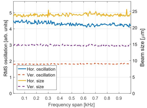
Figure 2: Bunch RMS oscillation and size as function of sweep frequency span. The measurement was conducted at a constant excitation frequency of 115.9 kHz (corresponding to the leftmost peak for this measurement), a sweep period of 100  $\mu$ s and an excitation amplitude of 0.1.
