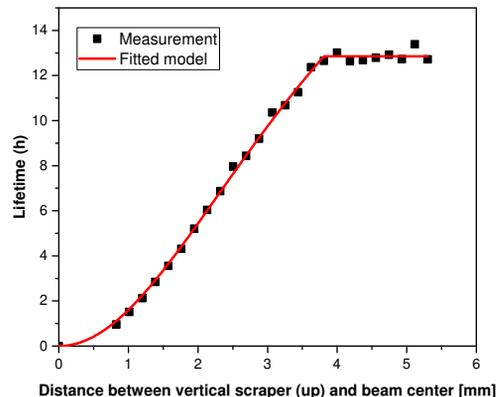
Figure 1: Lifetime vs. distance between the vertical scraper and the beam centre for tuned Landau cavities.
