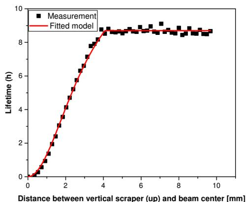
Figure 2: Lifetime vs. distance between the vertical scraper and the beam centre for detuned Landau cavities.
