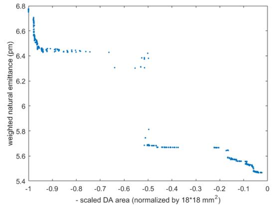
Figure 5: Final solutions after several iterations of PSO and MOGA for the HEPS booster.
