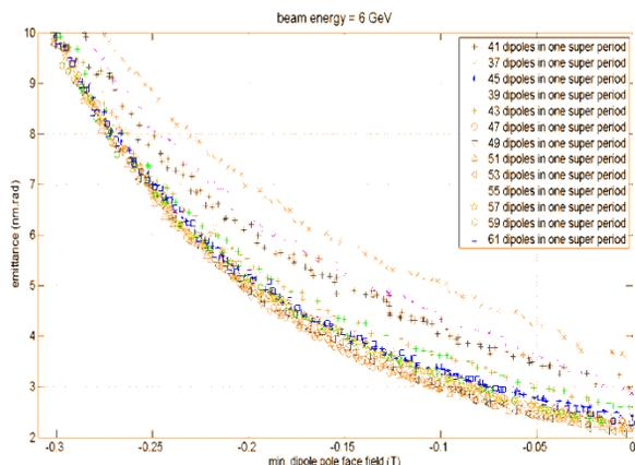
Figure 2: Variation of the available emittance with respect to the minimum dipole pole face field, for different numbers of dipoles in one super-period, obtained from PSO optimizations based on analytical expressions.
