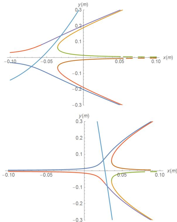
Figure 3: The pole face profiles of BF (upper) and BD (lower) for the HEPS booster, with  $y_0 = 14$  mm.
