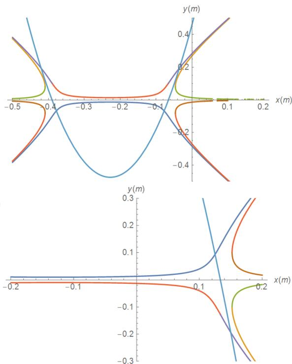
Figure 4: The pole face profiles of BF (upper) and BD (lower) for the NSLS-II booster, with  $y_0 = 14$  mm.
