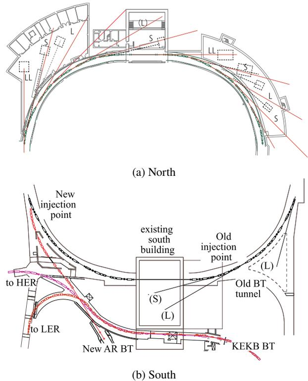
Figure 5: Beamline configuration for the existing experimental hall. “LL” shows the straight line from the about 20 m (B-B) straight section at the symmetrical point of the ring, “L” 2.7 m straight section at the arc and “S” 1.68 m. (a) shows the north side of the ring and (b) south.
