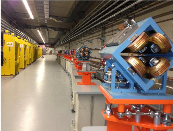
Figure 2: The FLASH2 tunnel (in beam direction) with the FLASH2 undulators to the left and magnets/magnet supports for the FLASHForward experiment in the FLASH3 beamline to the right.
