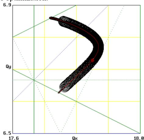
Figure 1: RF-steering: Tune variation. The red dot is the nominal working point and the radius of the circles corresponds to the actual beam current.
