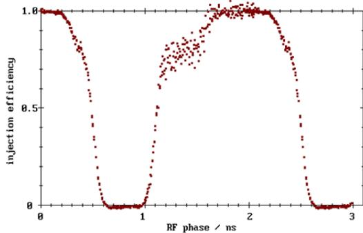
Figure 2: Impact of the RF-phase on the injection efficiency with on-axis injection and non-optimized sextupole settings.
