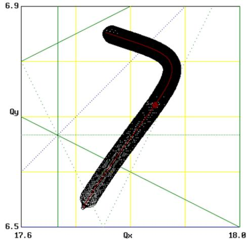
Figure 4: Tune variation by RF-steering: The  $Q_x+2Q_y$ -resonance can be crossed without losing beam. The width of the curve is proportional to the actual beam current.
