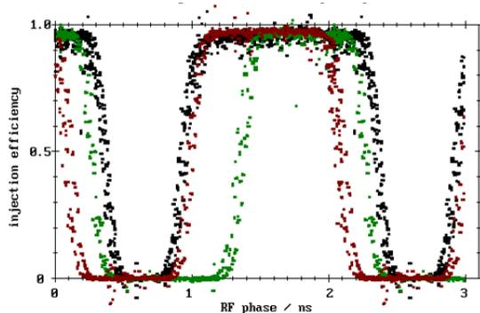
Figure 6: Phase acceptance for optimized sextupole settings and total accelerating voltages of 600, 1170 and 2100 kV (red, black and green).
