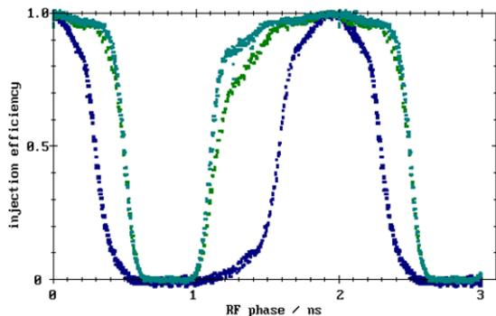
Figure 3: Accumulation efficiency as a function of the RF-phase with off-axis injection and non-optimized (blue) and after first and second optimization of sextupole settings (green and light blue).
