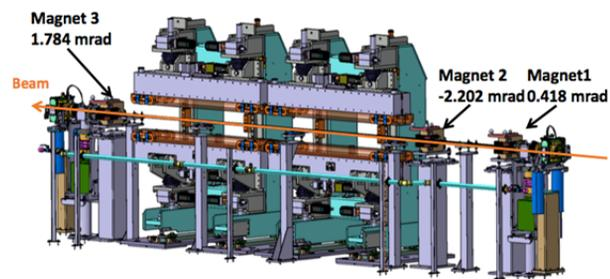
Figure 3: Electromagnetic 3-magnet chicane for the soft X-Ray BL TEMPO in order to use the femtosliced beam on axis.
