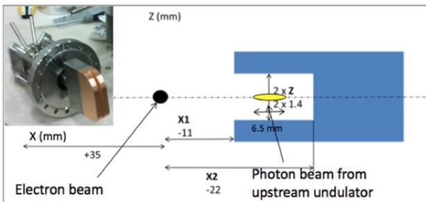
Figure 2: Dedicated movable photon absorber in 90-degree U-shape to block out any off-axis radiation from the upstream IVU.
