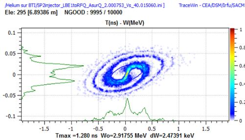
Figure 5: TraceWin simulation of a 0.15 mA He beam at the BEM location (see green projection on x-axis).
