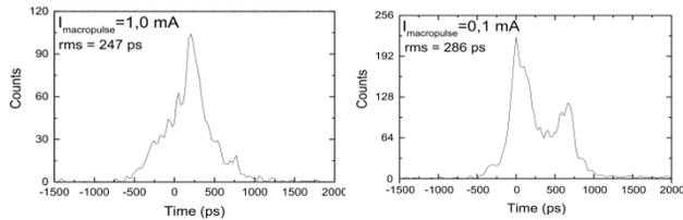
Figure 4:  ${}^4\text{He}^{2+}$  longitudinal bunch shape for 1 and 0.1 mA.
