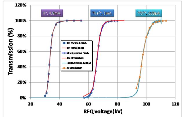
Figure 3: Comparison between measurement and TraceWin/Toutatis simulation (p, He and O beams).
