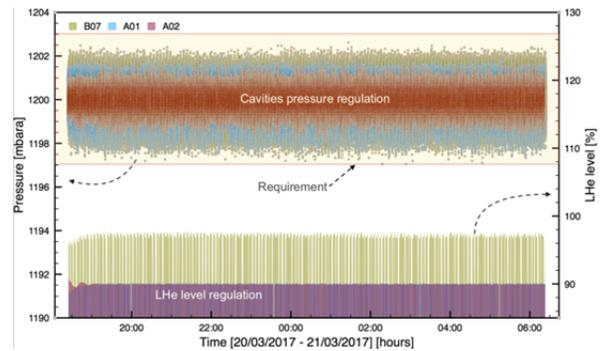
Figure 7: Pressure and liquid helium regulation for 3 cryomodules A01, A02, B07.
