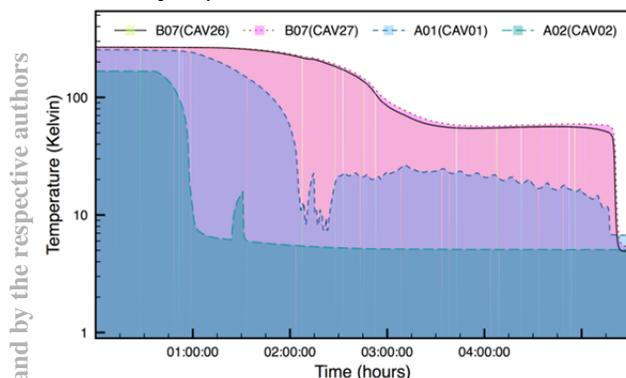
Figure 6: Cool down of the 4 cavities.
