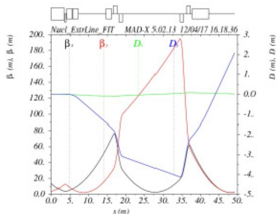
Figure 2: Optical functions of existing initial part of channel for applied researches.
