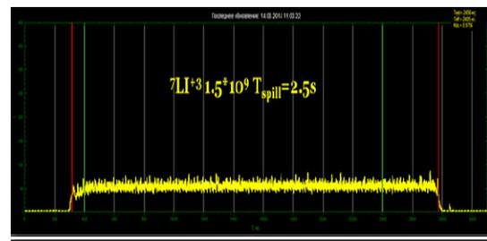
Figure 1: Example of the slow extraction beam spill.
