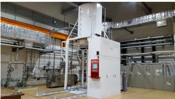
Figure 6: Vacuum brazing furnace.
