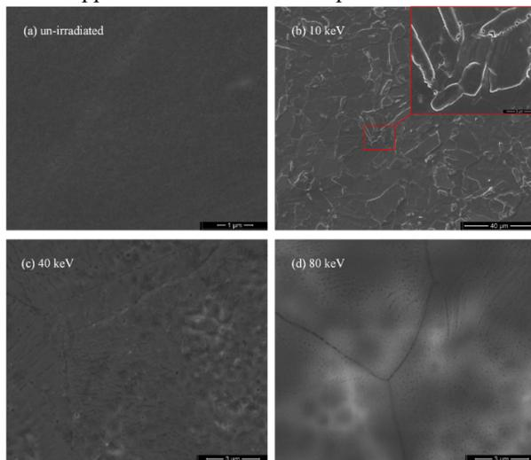
Figure 4: SEM images showing the copper samples (a) prior to irradiation and after irradiation energy of (b) 10 keV, (c) 40 keV, and (d) 80 keV.
