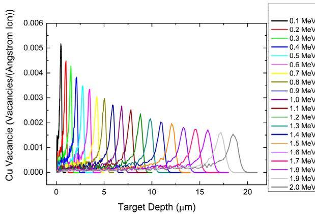
Figure 1: Depth distributions of vacancies in copper target correspond to normally incident proton beams with different energies from 100 keV to 2 MeV.
