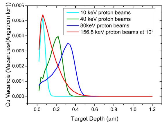
Figure 3: Depth distributions of vacancies in copper target correspond to normally incident proton beams with three different energies and the 156.8 keV proton beams at 10° glancing incidence.
