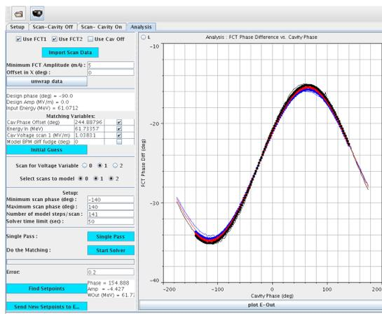
Figure 3: Phase scanning for LRBT debuncher cavity.
