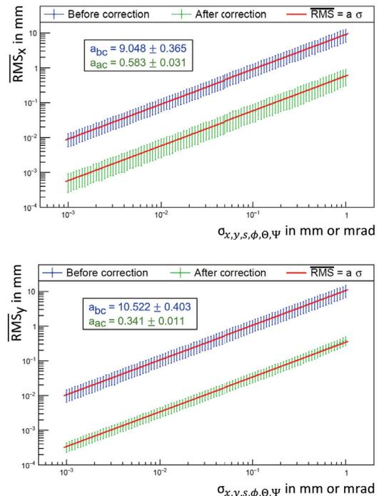
Figure 1: Mean closed orbit RMS in horizontal and transverse direction for simultaneous displacement and rotation of dipoles and quadrupoles. Blue markers: results before orbit correction. Green markers: results after the orbit correction. The values result from generating magnet misalignments using 1000 random seeds.
