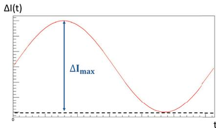
Figure 4: Sketch of sinusoidal residual power supply oscillation. The typical frequency of the power supply oscillation is approximately 600 Hz.
