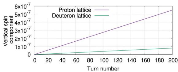
Figure 3: Average vertical spin components for 8 particles uniformly distributed on a vertical invariant of 0.1 mm mrad, as a function of the turn number, in a lattice with vertical closed orbit.
