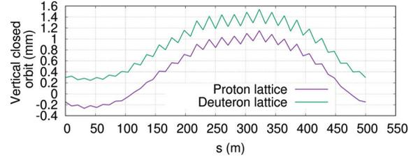
Figure 2: Vertical closed orbit along the ring for the proton and deuteron lattices.
