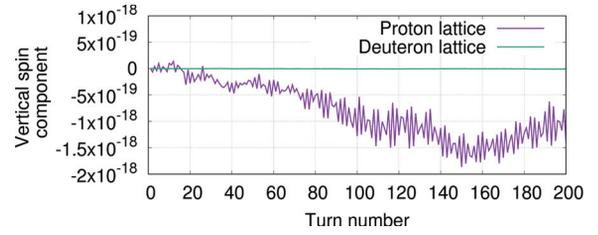
Figure 1: Average vertical spin components for 8 particles uniformly distributed on a vertical invariant of  $10^{-7}$  mm mrad, as a function of the turn number.
