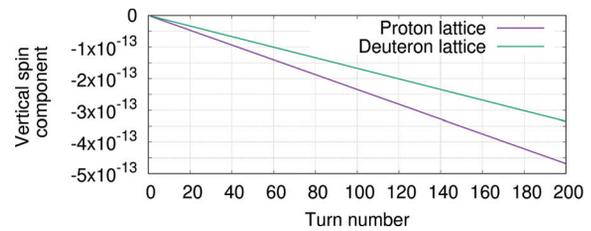
Figure 4: Average vertical spin components for 8 particles uniformly distributed on a vertical invariant of 0.1 mm mrad, as a function of the turn number, with an EDM of  $\eta = 10^{-15}$ .
