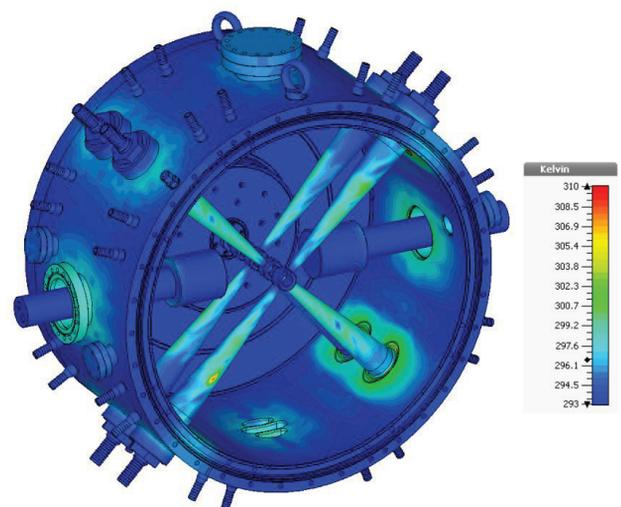
Figure 2: Simulated heat distribution at 5 kW input power [2]. The hottest spots, which are artifacts, heat up by 17 °C.
