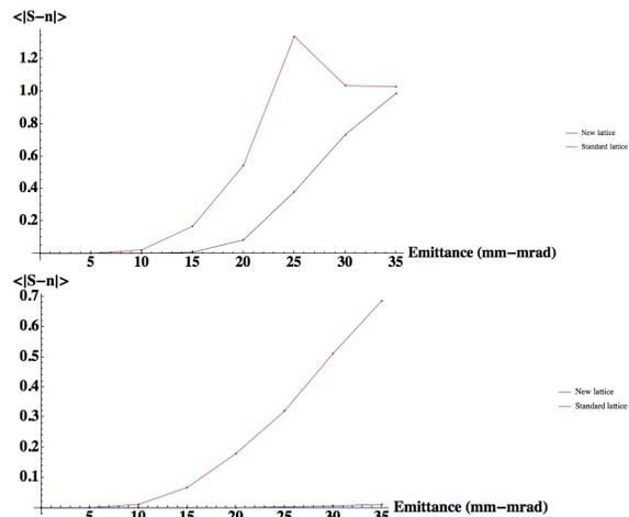
Figure 4: Polarization Transmission aperture for Blue (top) and Yellow (bottom) lattice. Each trace represents the amount of net difference between the stable spin direction and spin after crossing the  $G\gamma = 393 + Q_y$  spin resonance. This amount is calculated for each emittance. This shows the improvement compared to the old standard lattice.
