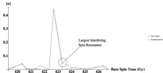
Figure 3: Calculation of intrinsic spin resonance strength at an emittance of 10 mm-mrad, near the strongest intrinsic spin resonance on the 255 GeV ramp ( $G\gamma = 393 + Q_y$ ). The calculations are for two lattices: the standard (old) lattice and the new lattice. Note the reduction of the neighboring resonances in the new lattice (largest one is circled).
