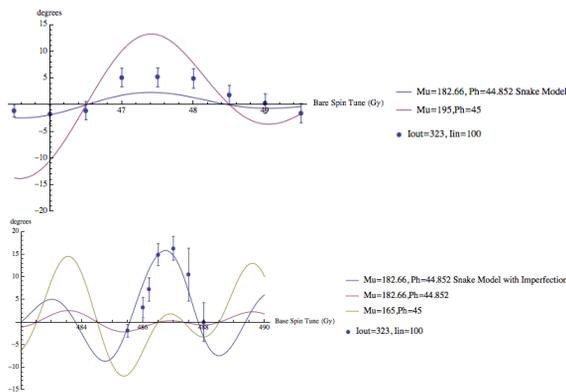
Figure 5: Energy scans of the projection of average spin tilt into horizontal plane at Injection (top) and at store (bottom) in Blue ring. We compared response to simple model with snakes at settings based on model value for  $I_{in}=100$  and  $I_{out}=323$  amps and with detuning of snakes and a strong imperfection source at  $G\gamma = 487$  (0.25).
