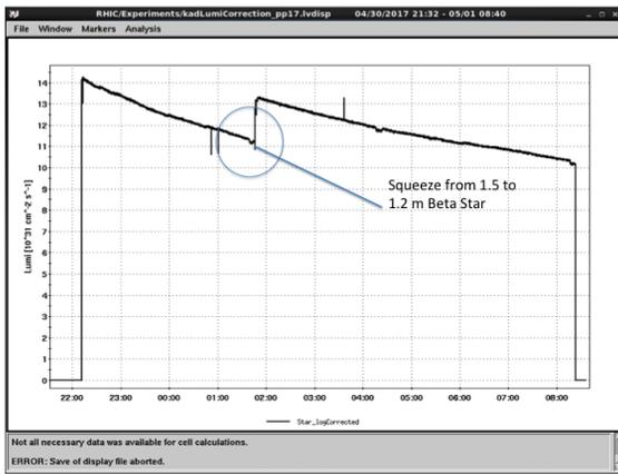
Figure 2: Luminosity Response to squeeze from 1.5 to 1.2 meter Beta Star.
