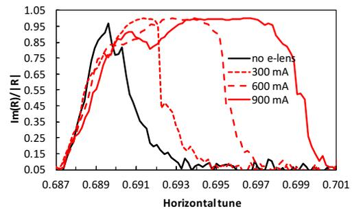
Figure 4: Measured p beam tune distribution width as a function of  $I_e$  without beam-beam collisions and with  $\sigma_e = 0.55$  mm. Curves are aligned to the left [1].
