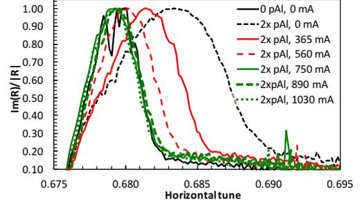
Figure 7: Tune distribution width reduction with the electron lens, measured in the proton beam with p+Al collisions.
