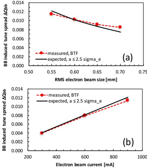
Figure 6: Measured and calculated increase in the tune spread in a  $\sigma_e$  scan (a) and a  $I_e$  scan (b). The calculation is for an amplitude range  $a$  from zero to  $2.5 \sigma_e$ .
