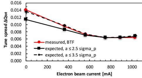
Figure 8: Total tune spread  $\Delta Q_{tot}$  as a function of the electron beam current  $I_e$ .
