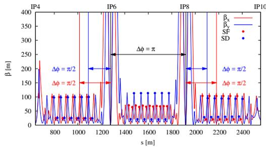
Figure 1: RHIC Blue ring ATS lattice for 100 GeV protons. Only a fraction of the 3.8 km circumference is shown.
