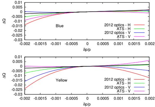
Figure 2: Blue (top) and Yellow (bottom) non-linear tune dependence on the momentum deviation  $\delta p/p$  for the 2012 lattice and the 2015 ATS optics. The black line in both plots corresponds to a linear chromaticity  $Q' = +1$ .
