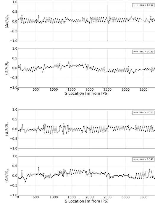
Figure 3: Measured  $\Delta\beta/\beta$  for the Blue (top) and Yellow (bottom) horizontal and vertical planes.
