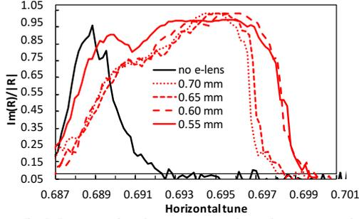
Figure 5: Measured p beam tune distribution width as a function of  $\sigma_e$  with  $I_e = 900$  mA.
