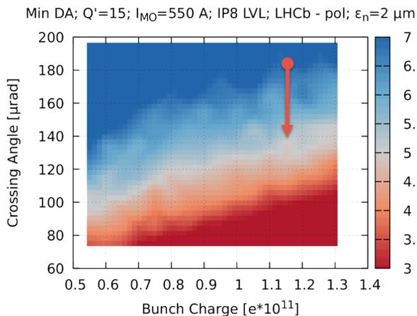
Figure 3: DA response to bunch intensity and crossing angle. The arrow indicates the crossing angle reduction performed during 2016. The DA at the beginning of the fill has been reduced to 5  $\sigma$ , the intensity decay gives more margin later in the fill.
