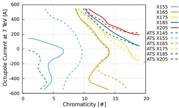
Figure 5:  $6\sigma$  DA boundaries in the chromaticity-octupole space, comparing the performances of Nominal and ATS optics for several crossing angles in IP1 and IP5. The legend indicates the half crossing angle values in  $\mu\text{rad}$ .
