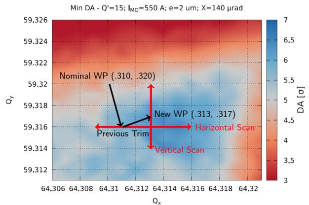
Figure 4: A tune scan showing that the performed adjustment to the tune. The arrows represent the area explored experimentally, carefully monitoring the beam lifetime.
