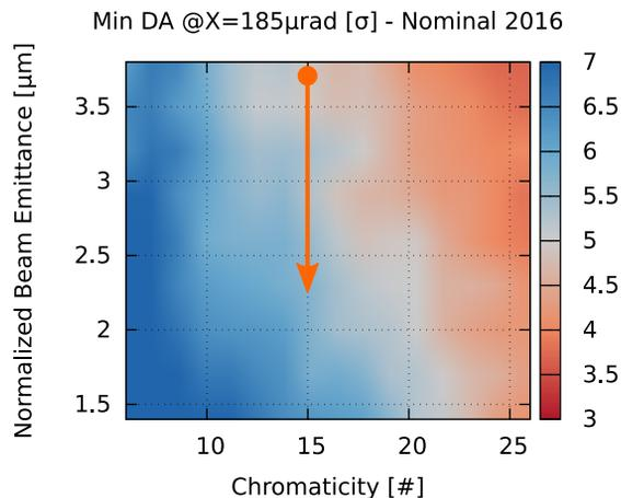
Figure 1: The additional DA gained for small emittances allows to run with higher chromaticity and/or with smaller crossing angle (not shown). The arrow indicates the reduction performed in 2016.
