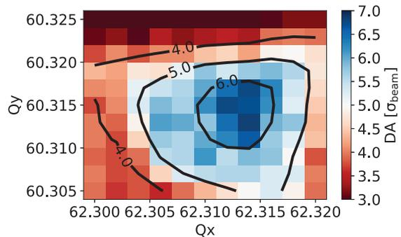
Figure 6: Tune scan for the proposed 2017 settings at collision. Good DA is obtained moving closer to the diagonal, provided that linear coupling is properly corrected.
