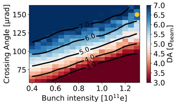
Figure 7: A Crossing-Intensity scan for the 2017 settings and optimised tune. The yellow dot is the proposed starting point for 2017, which is expected to give substantial margin.
