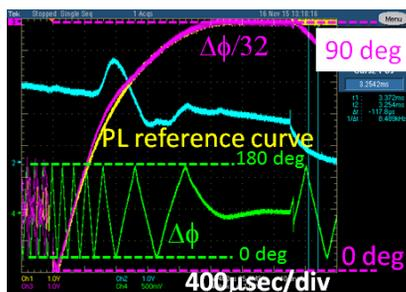
Figure 2: Illustration of the slow phase lock signals.
