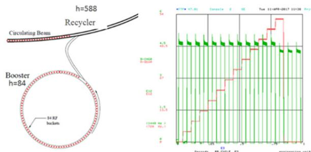
Figure 1: Illustration of beam delivery to the Recycler and beam intensities in the Booster (green) and Recycler (red).
