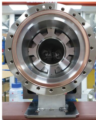
Figure 1: An inside view of the partially completed cavity assembly. The waveguide structures of the port couplers are clearly seen.
