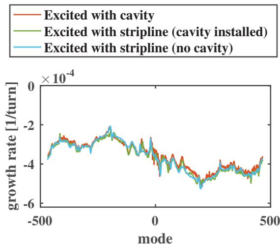
Figure 8: Comparing new cavity to stripline based test system, and assessing impact of the unpowered cavity on the synchrotron.
