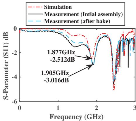
Figure 4: Representative bench measurements. There is broad agreement between simulation and measurements. The change due to bake out implies that the lower frequency discrepancy is due to fine detail in the waveguide coupler.
