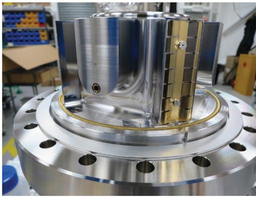
Figure 3: View of the internal structure of the cavity. The gold coloured components are for ensuring good RF continuity, while the silver ring is for the vacuum seal.
