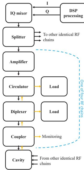
Figure 6: System diagram for the amplifier chains in the final configuration. Currently only I is driven.
