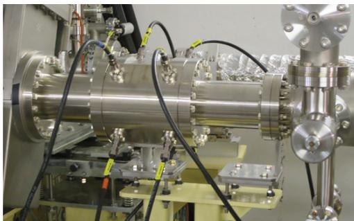
Figure 5: The kicker cavity installed in the storage ring. Upstream is left, downstream is right.
