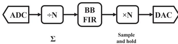
Figure 7: High level schematic of the LMBF DSP processing chain. After the signals are digitised the data for each individual bunch is decimated using a sum function. The data is put through bunch specific FIR filters. Then a sample and hold function increases the data rate to that which the DAC is expecting.
