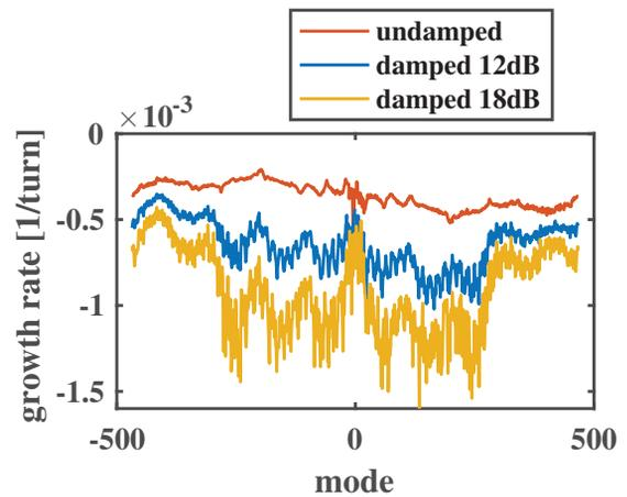
Figure 9: Feedback performance at different gains.
