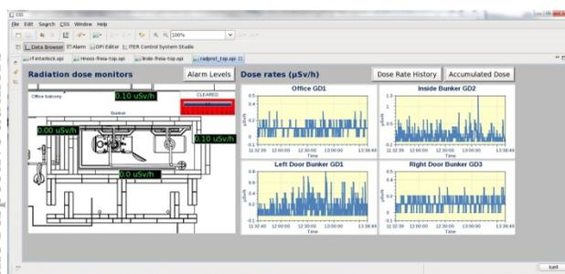
Figure 5: EPICS status display for the FREIA bunker showing the radiation monitors with graphs of dose rate, warnings messages- and clearing status.
