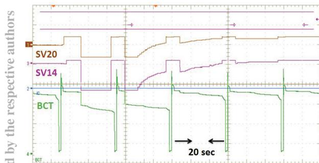
Figure 3: Exemplary oscilloscope screenshot during orbit correction. The green (lower) graph shows the beam current as function of time, indicating several machine cycles. In purple and brown the current through two vertical corrector magnets, namely SV20 and SV14 is displayed. Whereas the first cycle shows a regular ramp, during cycle number two the correction starts indicated by a step wise adjustment of the corrector current.
