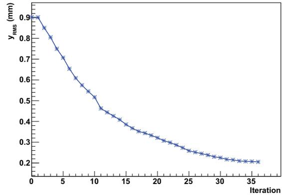
Figure 4: Correction of an artificially created local orbit bump. The rms of the vertical closed orbit distortion with respect to the initial orbit is displayed as function of the number of applied orbit corrections.
