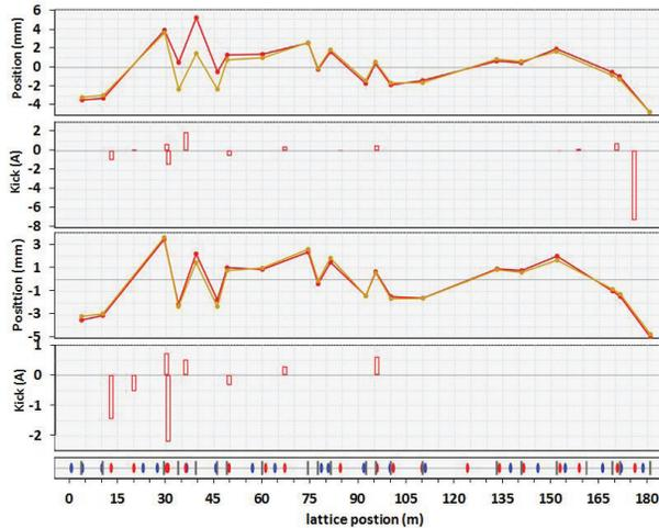
Figure 2: Detail of the graphical user interface, showing the present and the golden orbit and the set current of corrector magnets. In the upper panel a local three corrector orbit bump (red) was introduced with respect to the reference orbit (orange). The lower panel shows the orbit after correction, which is in good agreement with the reference orbit.
