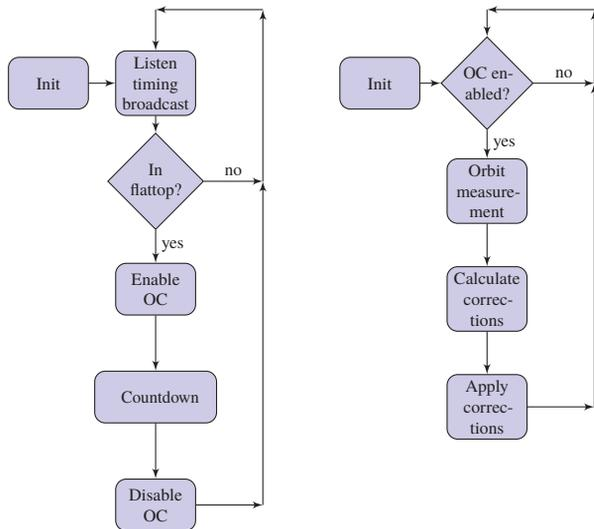
Figure 1: Block diagram of the orbit cycle control (left) and the orbit correction algorithm (right).
