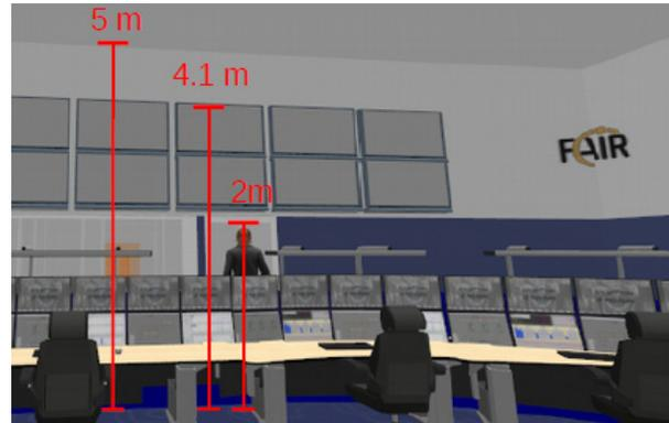
Figure 3: Planned FCC console, screen and fixed-display layout in relation to the control room's reference ceiling height.
