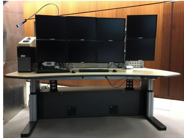
Figure 5: First generation prototype height-adjustable standing console.
