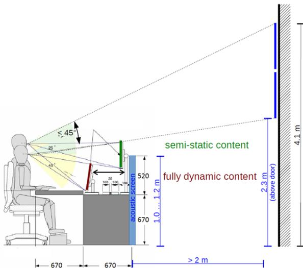
Figure 4: Nominal console and screen geometry in relation to fixed-displays and required distances, based in part on earlier CCC design described in [10].
