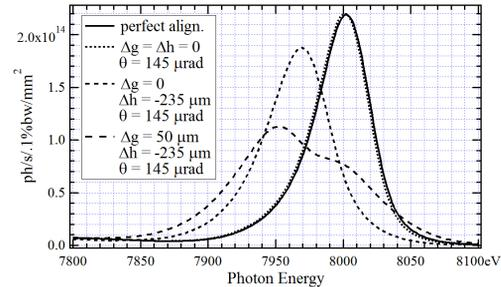
Figure 2: Calculated on-axis spectral flux per unit surface at  $\sim 33$  m observation distance at 5th harmonic of perfectly aligned IVU of SRX beamline (solid line) and for different cases of misalignment (dotted / dashed lines).
