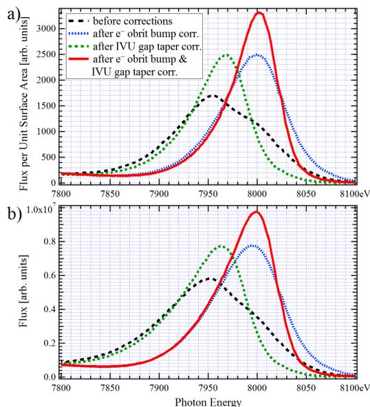
Figure 4: UR measured at 5th harmonic of IVU at the SRX beamline before and after applying electron orbit “bump” and undulator gap taper corrections: a) on-axis spectral flux per unit surface area; b) spectral flux within  $\sim 40 \times 40 \mu\text{rad}^2$  aperture (used for experiments at SRX).
