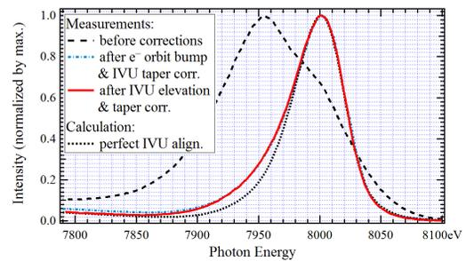
Figure 5: On-axis UR spectral flux per unit surface area at 5th harmonic of SRX IVU, measured before and after spectrum based alignment by two different methods, compared to calculation made for perfectly aligned IVU.
