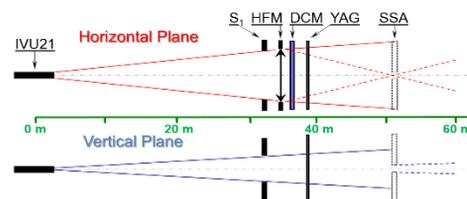
Figure 3: Optical scheme of the SRX beamline initial part.
