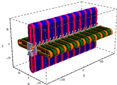
Figure 3: Possible SCAPE configuration with racetrack coils and magnetic poles.
