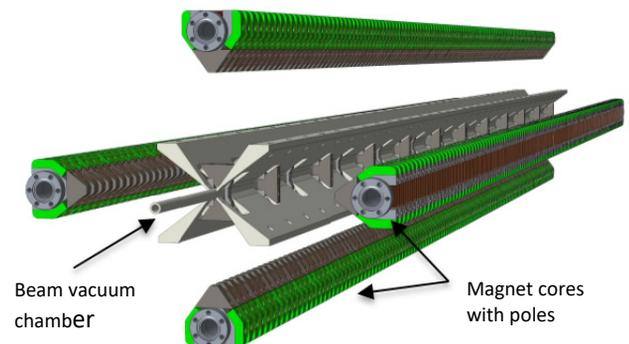
Figure 5: Exploded view of SCAPE magnet with a beam chamber.
