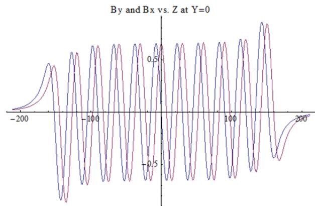
Figure 2: Simulated SCAPE magnetic field profiles in vertical plane (blue) and horizontal plane (red). Vertical axis is in T, and horizontal axis is in mm.
