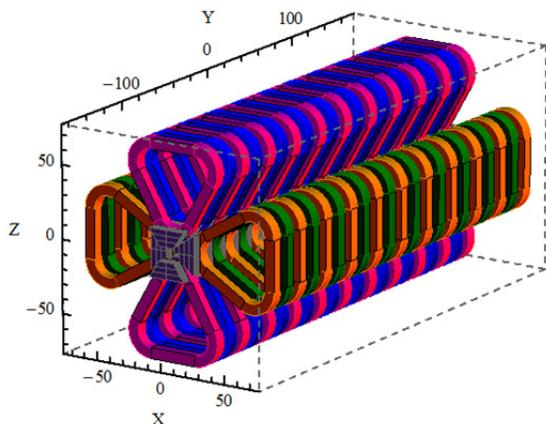
Figure 4: SCAPE configuration with recessed triangular coils and magnetic poles.
