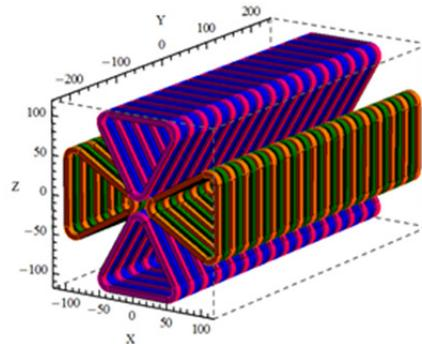
Figure 1: Concept of SCAPE— a universal SCU with four planar superconducting coil structures. A round beam chamber is not shown.
