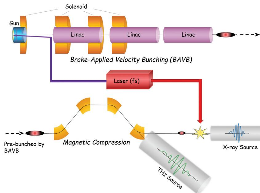
Figure 3: Design of THz/X-ray sources for pump-probe experiments.
