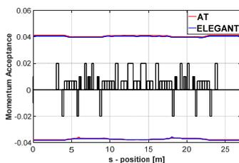
Figure 1: The momentum acceptance for the HEPS storage ring.
