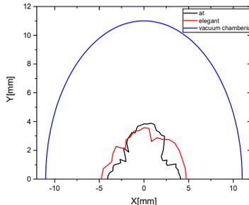
Figure 4: Dynamic aperture and physical aperture at the centre of the long straight section.
