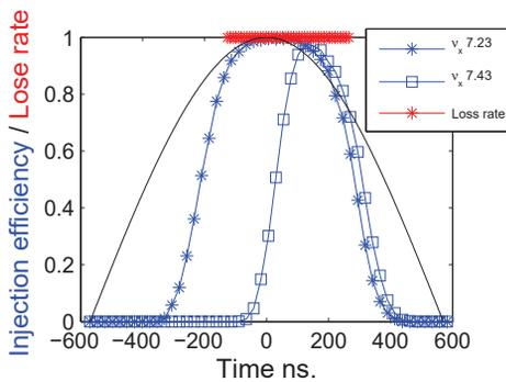
Figure 6: Injection efficiency and loss rate for design and optimized tunes. 1 mrad. kick was used for simulation. Loss rate is calculated as the ratio between number of particle survived after 200 turns and initial number of particles.
