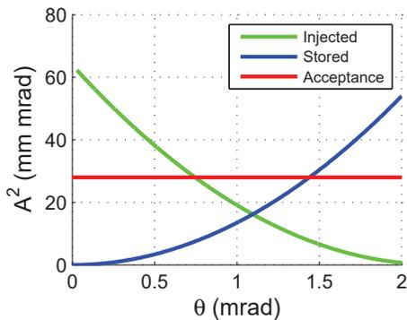
Figure 2: Normalized amplitudes of the injected and stored beam as a function of kicker strength at straight 5.
