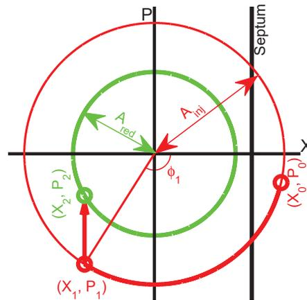
Figure 1: Motion of injected particle in normalized phase space.
