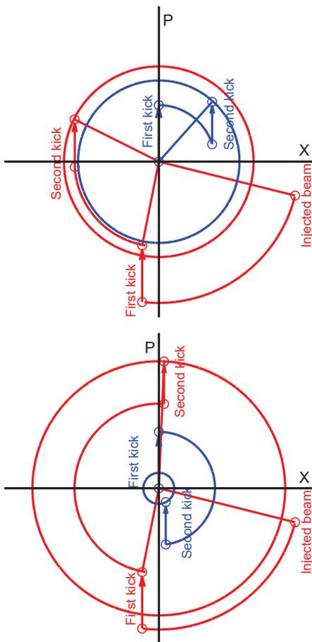
Figure 5: Visualization of injection process in normalized phase space. Top plot: design tune (7.23). Bottom: Optimized tune (7.44). Blue color is for stored beam and red for injected. Scales do not correspond to the real case. Pictures are for illustration purpose.
