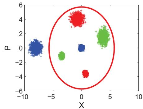
Figure 4: Normalized phase space of injected and stored beam for 1 mrad. kick at location 5. First 3 turns after injection are shown. Circles are the injected beam and crosses stored. Color code: Blue - first turn, Red - second, Green - third.
