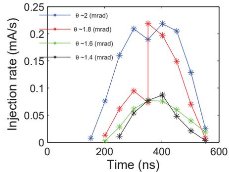
Figure 7: Accumulation rate as a function of injection timing for 4 different kicker strength.
