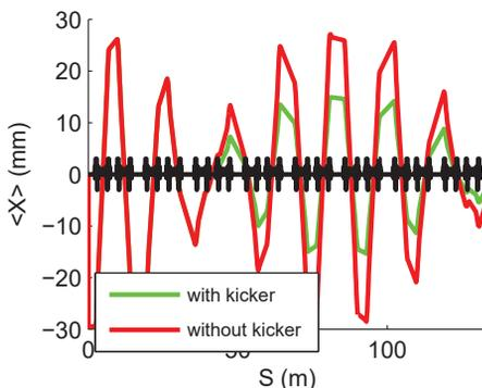
Figure 3: Trajectory of injected beam with and without kicker.
