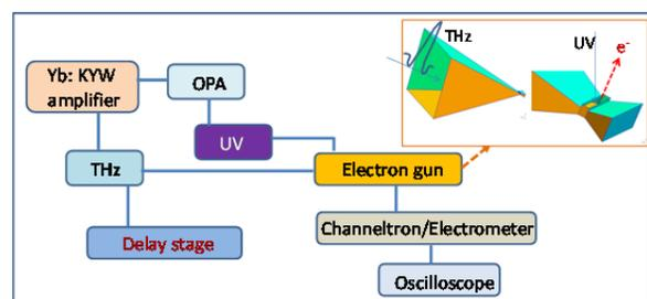
Fig.1: Schematic of the whole system of the electron acceleration in an ultrafast gun by THz pulses.
