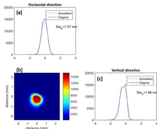
Figure 5: THz beam diameters at horizontal (a) and vertical (c) directions are 1.57 and 1.68 mm respectively. The
