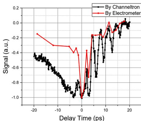
Figure 7: Electron signals measured by channeltron and by electrometer versus delay time between THz and UV pulses. Several peaks were observed during the scanning.
