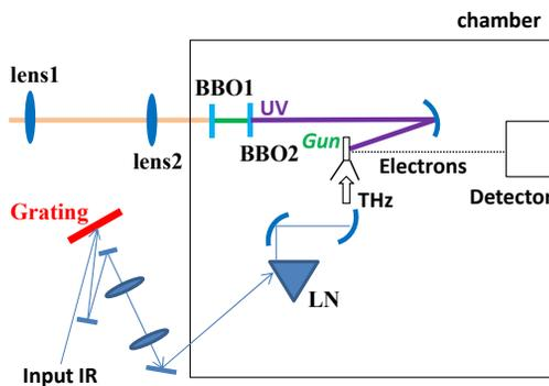
Figure 3: Schematic of THz generation and electron acceleration system.
