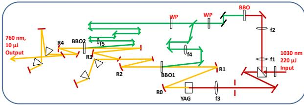
Figure 2: Schematic of the OPA generation system.
