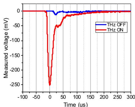
Figure 6: Measured voltage induced by accelerated electrons with THz OFF and ON.
