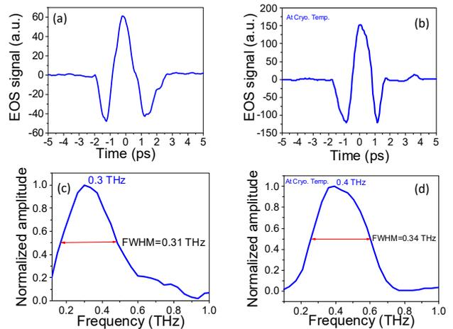
Figure 4: EOS traces and spectra at two cases: room temperature and cryo. Temperature. (a) EOS signal for the THz pulses at room temperature; (b) EOS signal for the THz pulses at cryo. Temperature; (c) Normalized amplitude of THz pulses in the frequency domain at room temperature. (d) Normalized amplitude of THz pulses in the frequency domain at cryo. temperature.
