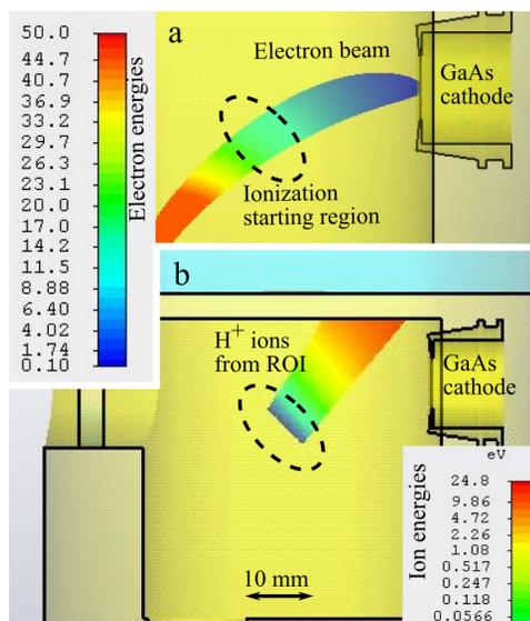
Figure 2: The region within the electrode chamber where the electron beam reaches sufficient energies to ionize molecular hydrogen (a). Ions originating from this ROI travel back on the bent field lines and miss the GaAs cathode (b), presuming they have no initial kinetic energy. Simulated with CST studio suite®.
