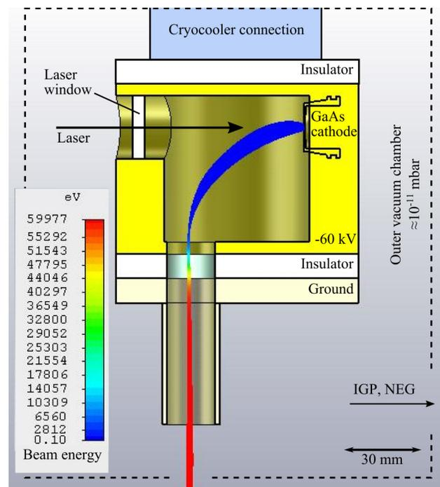
Figure 1: A first layout of the cryogenic source with simulated electron beam (CST studio suite<sup>®</sup>).
