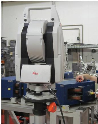
Figure 5: The lasertracker AT401 from Leica is shown during its operation for the alignment at the S-DALINAC.
