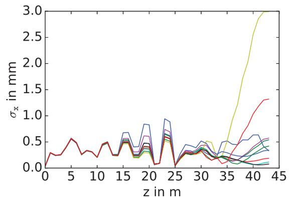
Figure 4: The one-sigma envelope in x-direction following the first recirculation for ten different misalignment settings is shown. An increase of the x-dimension of a factor of up to ten is possible until the end of the recirculation in comparison to an optimized lattice.
