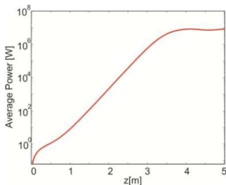
Figure 5: The SASE FEL radiation power along the undulator for 10  $\mu\text{m}$  radiation wavelength
