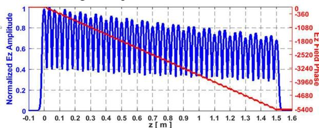
Figure 2: On-axis accelerating field along the AREAL travelling wave structure
