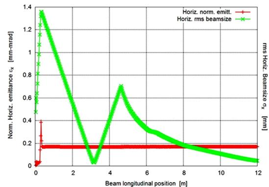
Figure 4: The beam size and normalized beam emittance evolution along the linac, without space charge.
