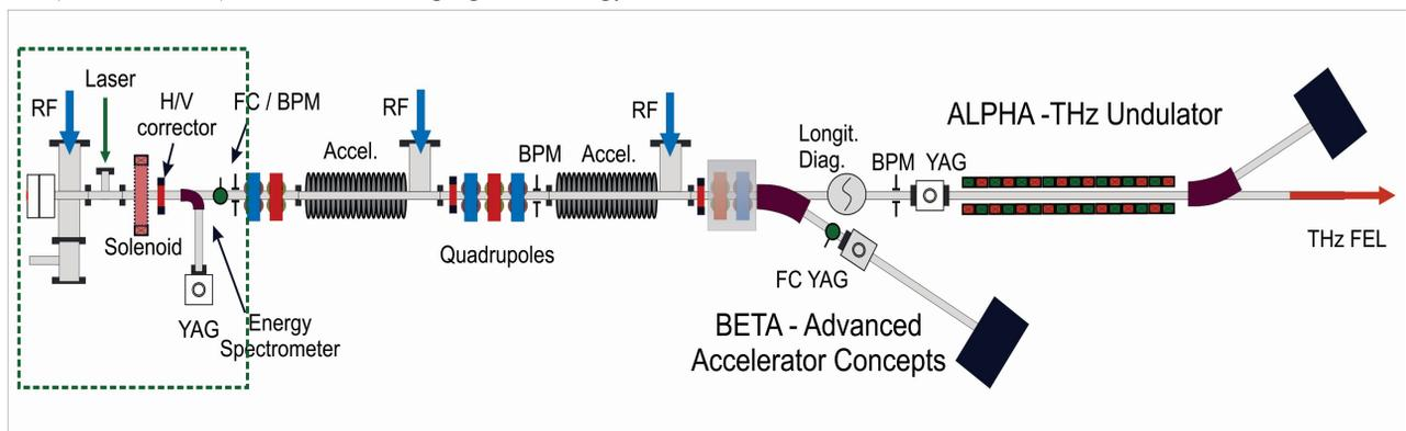
Figure 1: Schematic overview of existing (marked) and future upgrade parts of AREAL accelerator.
