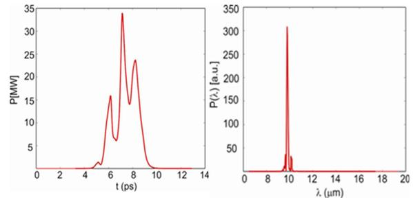
Figure 6: Power distribution along the bunch (left) and the radiation spectrum (right) at the saturation point for radiation wavelength of 10  $\mu\text{m}$ .
