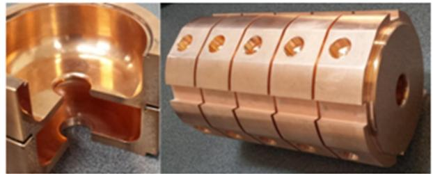
Figure 3: Brazing test with 2-cell (left) and 5-cell prototypes (right).
