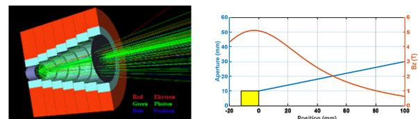
Figure 7: Schematic (left), the magnetic field and aperture (right) of AMD. The yellow block is target.
