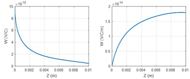
Figure 4: The short-range Wakefield of S-band accelerating tube, left is longitudinal Wakefield and right is transverse Wakefield.
