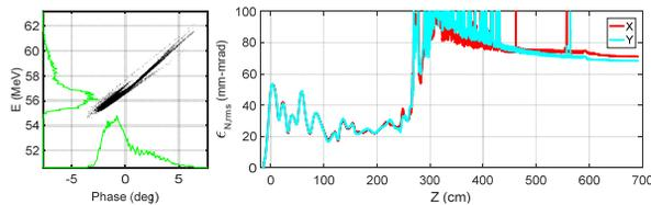
Figure 2: Beam distribution at exit of ESBS (left) and normalized rms emittance (right) along beam direction.
