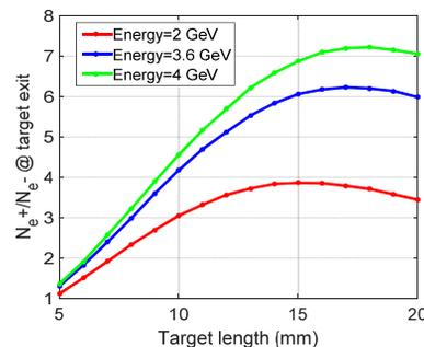
Figure 6: Positron yield with different target length and different electron energy.
