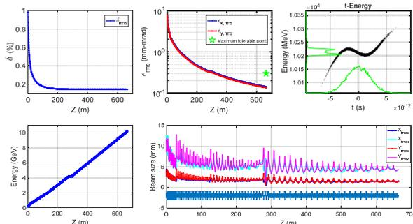
Figure 10: The simulation results along the linac: energy spread (top left), emittance (top middle), longitudinal phase space distribution (top right), energy (down left) and beam sizes (down right).
