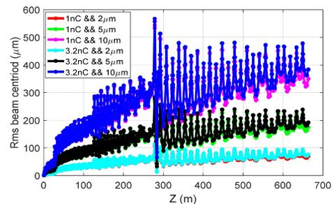
Figure 11: The vertical rms beam orbit jitter with different quadrupole vibration amplitude along the linac.
