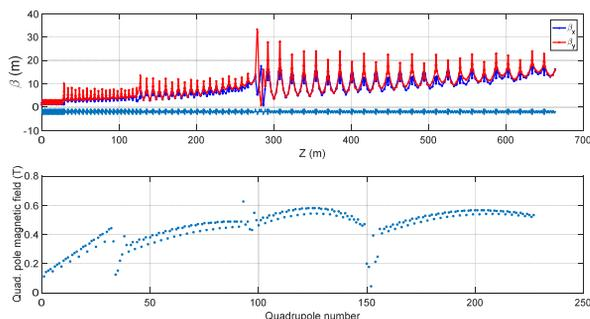
Figure 9: The  $\beta$  function and quadrupole pole magnetic field along the linac.
